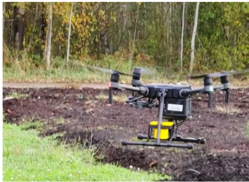
TGNR drone with leak detection technology
